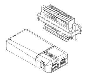
By means of the PSU kit, multiple LED lamps can be controlled simultaneously through a multiple connection board (9x3x5 cm) connected to a driver. In the event of a failure of even a single LED, the board allows the other LED to continue working properly.
